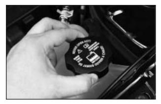
You can remove the coolant surge tank pressure cap when the cooling system, including the coolant surge tank pressure cap and upper radiator hose, is no longer hot. Turn the pressure cap slowly counterclockwise about one-quarter of a turn.
